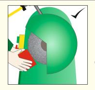
CORRECT - The work should be pushed gently against the rotating mop. It should be held firmly in both hands and moved continuously left and right, against the lower part of the mop.
