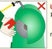
UNSAFE - The work is about to be pressed against the top part of the mop. This is dangerous, as the work will be 'ripped out' of the machine operators hands. It will fly at high speed, towards him/her.
