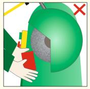
UNSAFE - This is a dangerous way to hold the work, as its top corner is about to be caught by the rotating mop. The work will be 'wrenched' from the machine operators hands.
